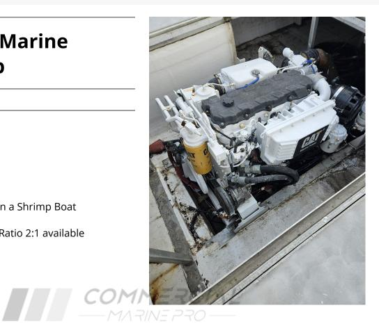
Categories: Marine Engines Cooling Method Heat Exchanger Engine Manufacturer/Brand CAT Engine Model C9.3 HP 567 RPM 2500 Condition RTO
