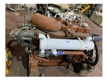
Categories: Marine Engines Cooling Method Heat Exchanger Engine Manufacturer/Brand Cummins Engine Model 6CTA HP 450 Condition Rebuilt Additional Information Pictured unit is of previously rebuilt/sold unit.
